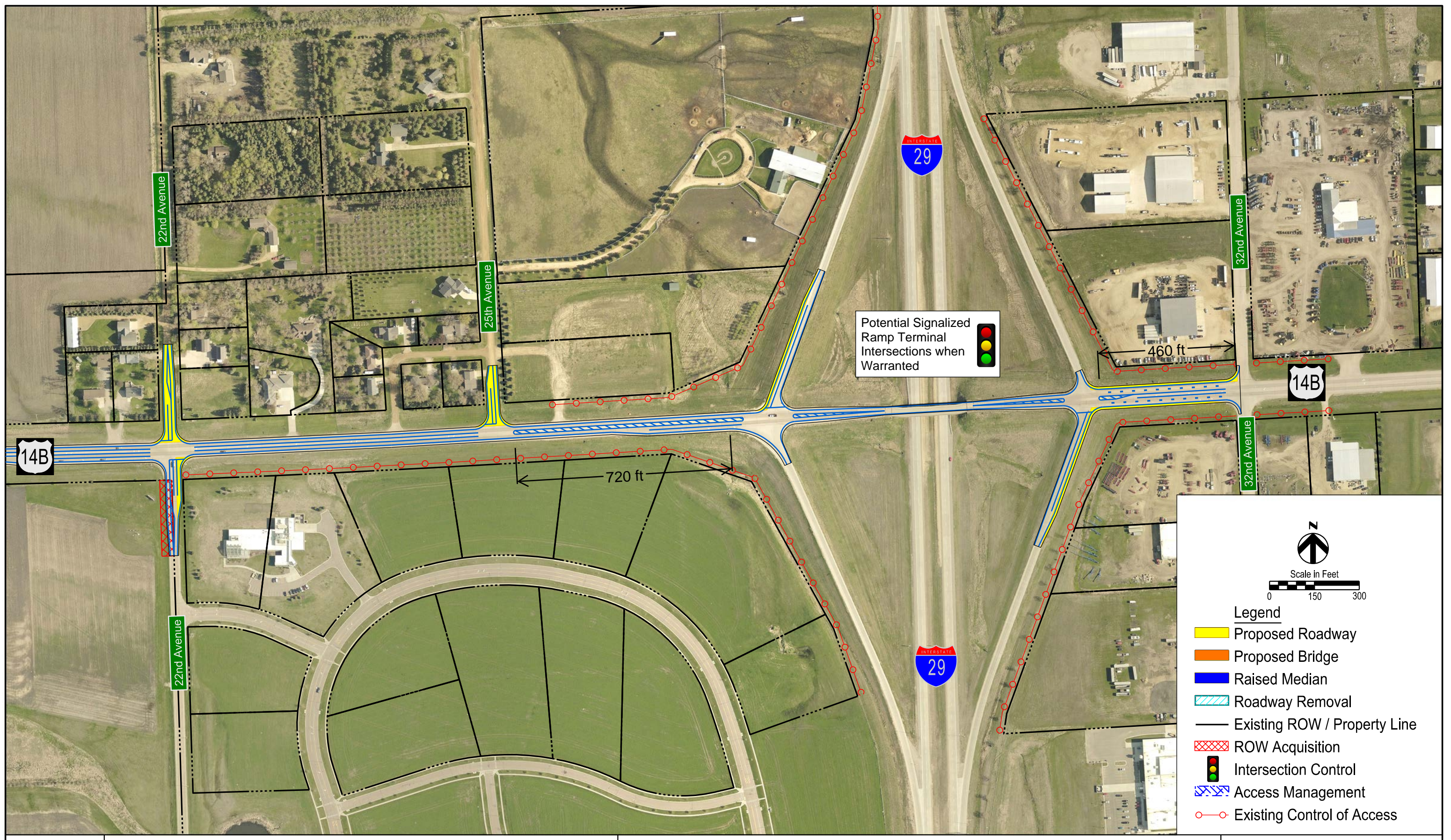
HR DOT brookings Volga U.S. Department of Transportation Federal Highway Administration US14 Bypass Concepts - I-29/US14 Bypass Interchange Option A: Improved Existing Diamond Interchange US14 / US14B Corridor Study Brookings, SD Figure I-29/US14 Bypass Interchange - Option A
